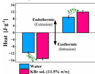
**Fig. 2** Intrusion and extrusion heats where exothermic in negative and endothermic in positive.
