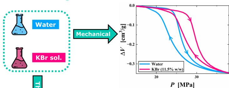
**Fig. 1** Compression (intrusion)/decompression (extrusion) PV-isotherms
