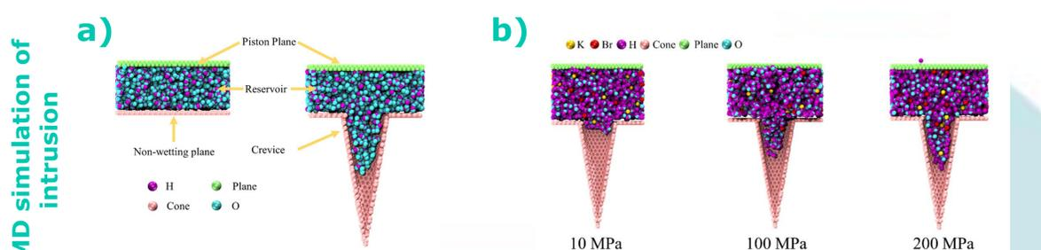
**Fig. 3 a)** Configurations to simulate intrusion where the first system consists of a liquid reservoir situated between two flat planes and the second system where a flat plane is transformed into a plane featuring a 2 nm diameter hole with a crevice (nano-cone). **b)** Snapshots of the Visual Modelcular Dynamics (VMD) for the intrusion of the KBr solution at 10, 100 and 200 Mpa.
