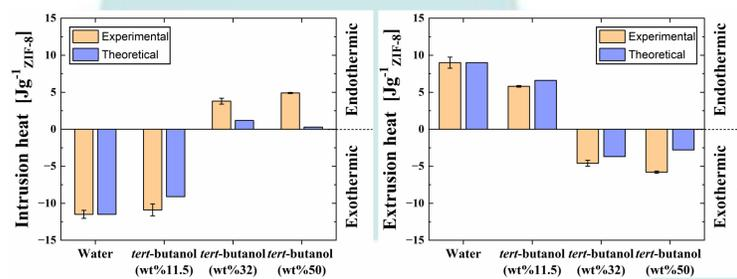
**Fig. 5** Thermal performance for {ZIF-8+ tert-butanol solution}.
