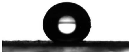
Figure 3.- Wettability test of 8<sup>th</sup> batch of grafted  $\text{CF}_3\text{-SiO}_2$  (FG150-EA8) by means of contact angle measurements.
